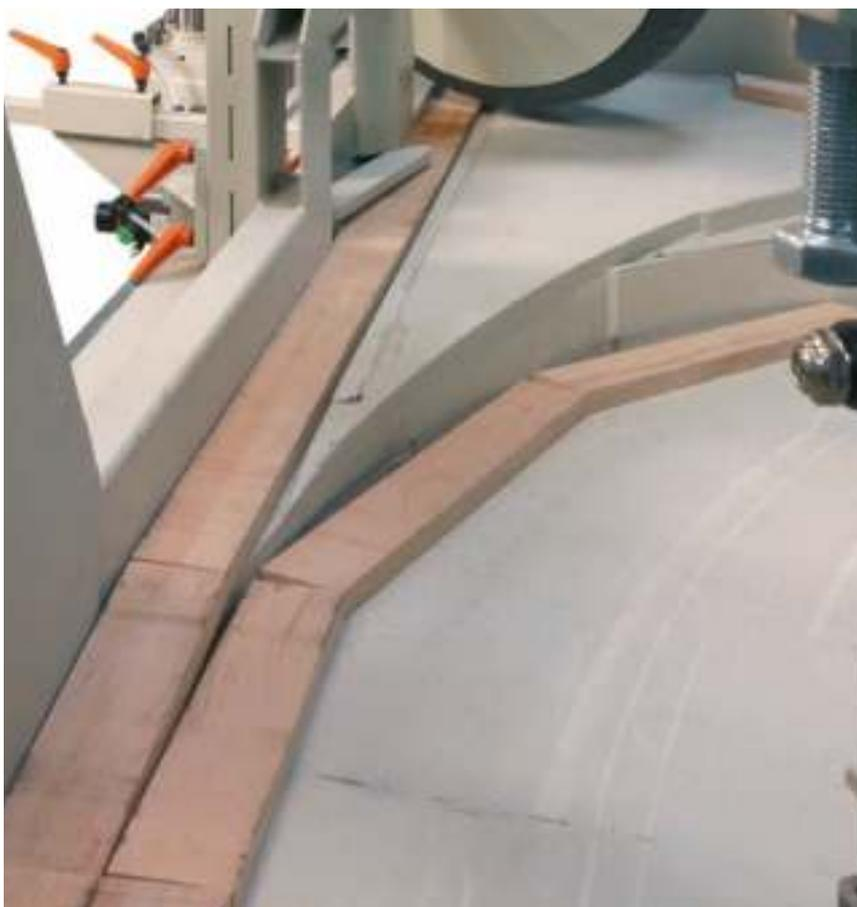
**The HS 200 Spinfeed** is the automatic alternative to any other highspeed feeding unit of a horizontal finger jointing line. The short timber pieces are automatically fed into the finger jointer, no matter whether they are initially coming from an optimizing cut-off saw or from a container.
